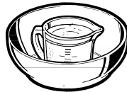
How to test for a microwave-safe dish.
