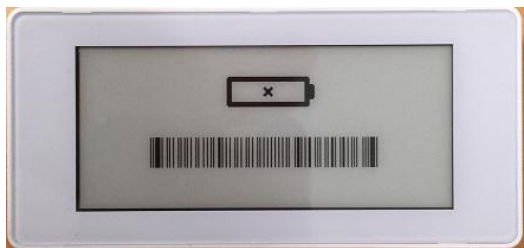
Battery is dis-charged (to need changing battery)
