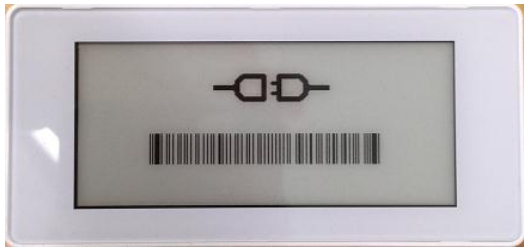
Disconnected to gateway
