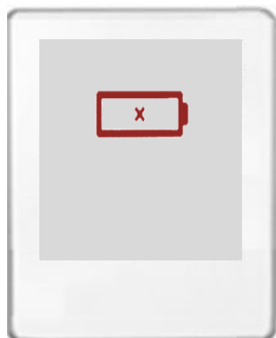
Battery discharge (The battery needs to be replaced)
