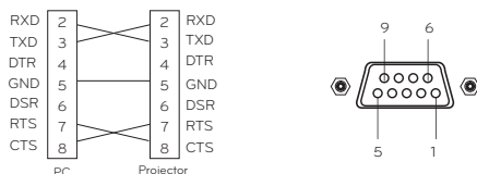
<Figure 1, RS-232 connection diagram>
