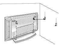
Secure the TV assembly to the wall with strong strings or wound wire cables, (not supplied with the product), as shown.
