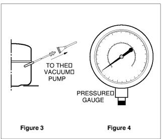
In case that a considerable leakage occurs and to stop the vacuum pump will be necessary and add a small quantity of Freon to the system, if vacuum should not be obtained (pressure gauge can't fall to 1 atmosphere.), start the refrigeration unit and find the leakage with the special leak-finder. When the defective soldering point is visible, re-do it after opening the extension tube valve and reestablishing the normal outside pressure inside the group.
