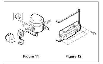
5. Remove the Compressor by loosening 2 earth screws next to Compressor.
