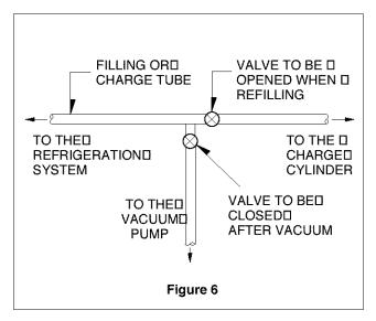
In addition, check the graduated scale on the cylinder for the quantity of R-12 to be added, for example, if we have 750 grams of Freon in the cylinder and must add 165 grams to the group, this amount will be reached when R-12 has dropped to 585 grams, remembering that the indicator shows a lower limit of meniscus. Do this after choosing the scale corresponding to the gas pressure different scales reported as the same gas pressure indicated by the pressure gauge on the top of the column.
