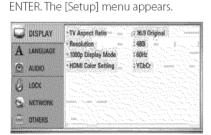
**3.** Use  $\Lambda/V$  to select a first setup option, and press > to move to the second level.
