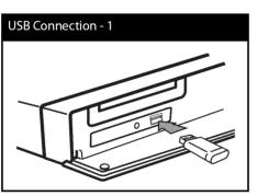
When you connect the USB device on the HOME menu, the player plays a music file contained in the USB storage device automatically. If the USB storage device is containing various types of files, a menu for the file type selection will appear.
