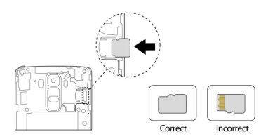
• Insert the microSD card all the way gently without bending and with the terminals facing down.
