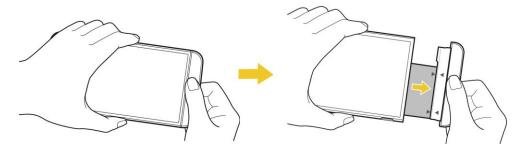
3. Hold the battery and module with both hands and separate them from one another in an outward arc (as indicated below) to disconnect the battery terminals.
