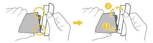
3. Push the battery module all the way into the device.
