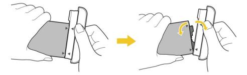
**Note**: This device is supplied with the battery inserted. When using the device for the first time, check the battery level and fully charge the battery before using the device if necessary.
