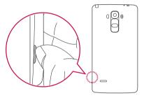
2 Slide the SIM card into the lower slot for the SIM card as shown in the figure. Make sure that the gold contact area on the card is facing downward.
