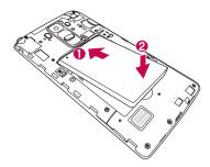
4 To replace the cover onto the device, align the cover over the back of the phone and press it down until it clicks into place 2.
