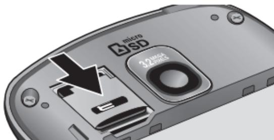
**! WARNING:** Do not insert or remove the memory card when the phone is on. Otherwise, it may damage the memory card as well as your phone, and the data stored on the memory card may be corrupted.
