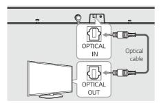
2. Select the input source to OPTICAL by pressing **F** button on the remote control or unit repeatedly.
