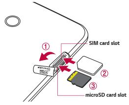
3 If you want to use a memory card, insert the memory card into the lower slot. Make sure the gold contact area is facing upwards. Slide the microSD card into the slot until it "clicks" into place and then close the slot cover.
