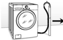
Connecting the drain line
