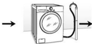
Connecting the drain line
