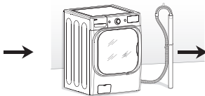
Connecting the drain line
