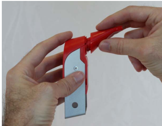
Figure 10: Removing the mouthpiece
