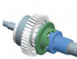
Quick Release gear without spline. Drawing no.: LA27QR_17
