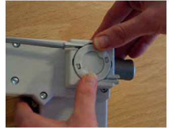
Fig. 3. Replacement of QR cover.
