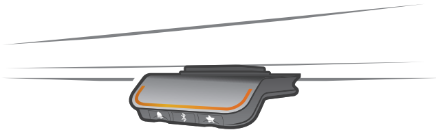
Figure 5: Pulsating orange light strip indicates the user needs to change position
