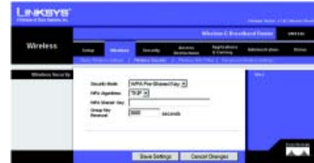
Figure 6-17: Wireless Tab - Wireless Security (WPA Pre-Shared Key)
