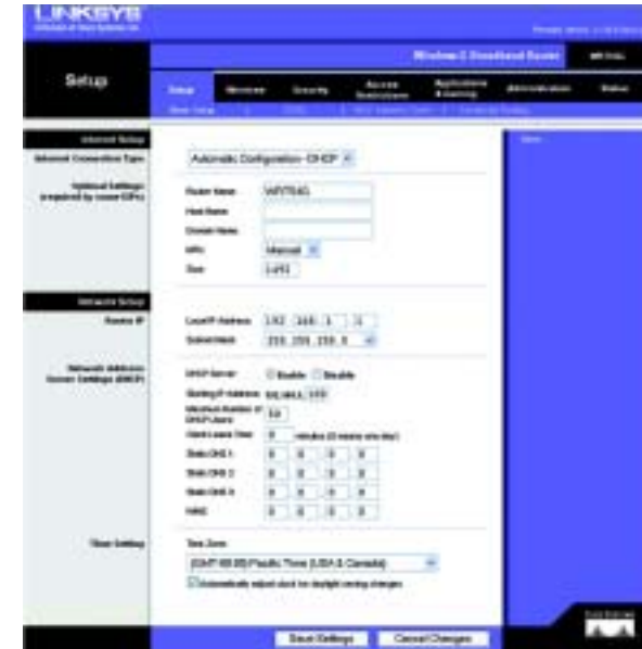
Figure 6-2: Setup Tab - Basic Setup
