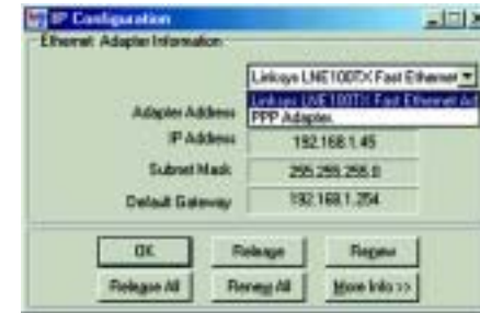
Figure E-1: IP Configuration Screen
