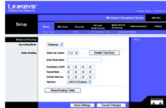
Figure 6-14: Setup Tab - Advanced Routing (Gateway)
