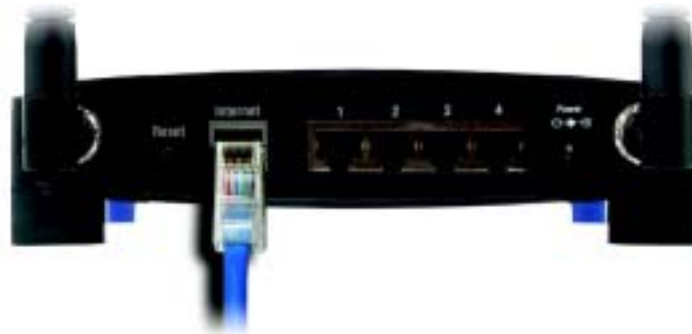
Figure 4-2: Connecting Your Internet Connection
