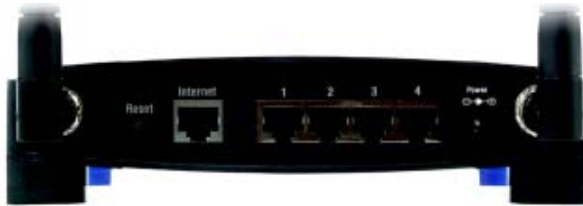
Figure 3-1: The Broadband Router's Back Panel
