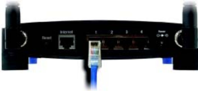
Figure 4-3: Connecting Your Network Devices
