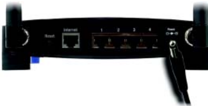
Figure 4-4: Connecting the Power
