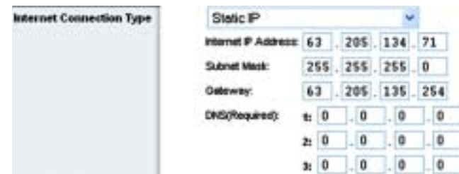
Figure 6-4: Static IP Connection Type
