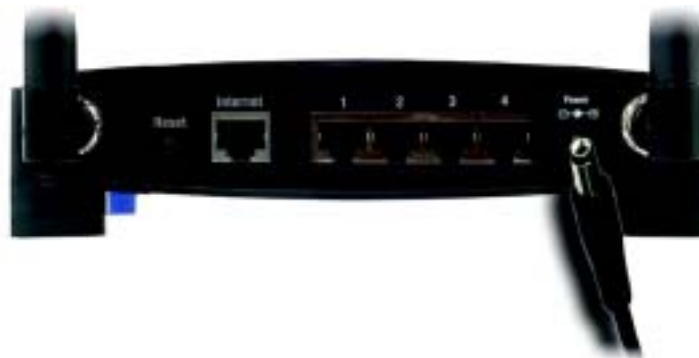
Figure 4-8: Connecting the Power
