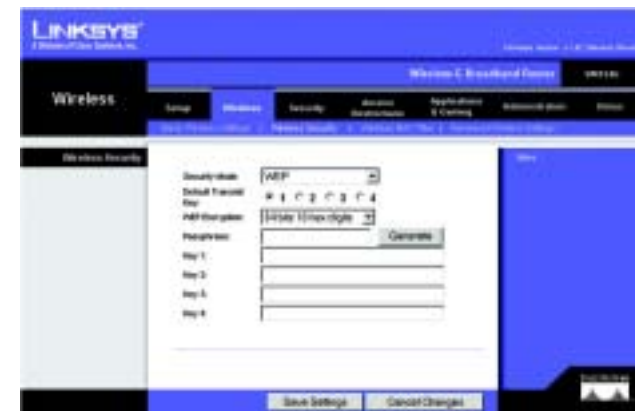
Figure 6-20: Wireless Tab - Wireless Security (WEP)
