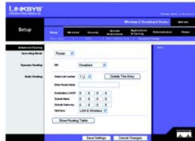
Figure 6-15: Setup Tab - Advanced Routing (Router)
