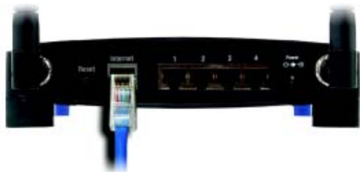
Figure 4-6: Connecting Another Router
