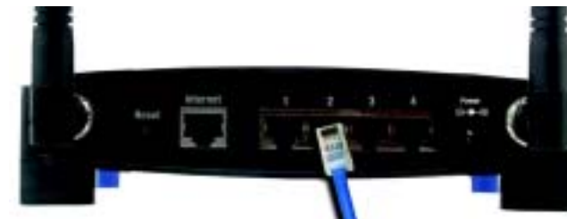
Figure 4-2: Connecting Your Network Devices
