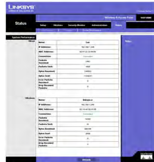
Figure 6-26: Status - System Performance
