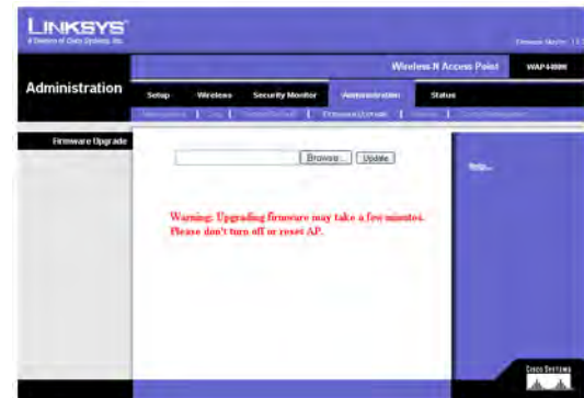
Figure 6-21: Administration - Firmware Upgrade
