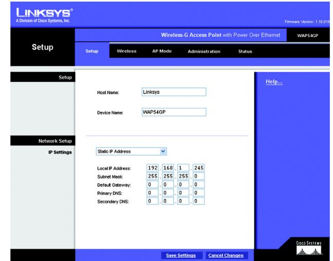
Figure 6-3: Setup - Static IP Address Screen
