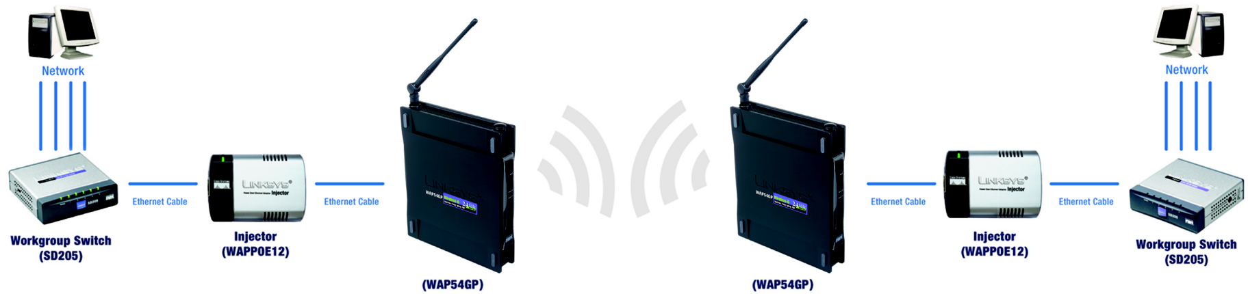
Figure 6-15: Wireless Bridge Diagram
