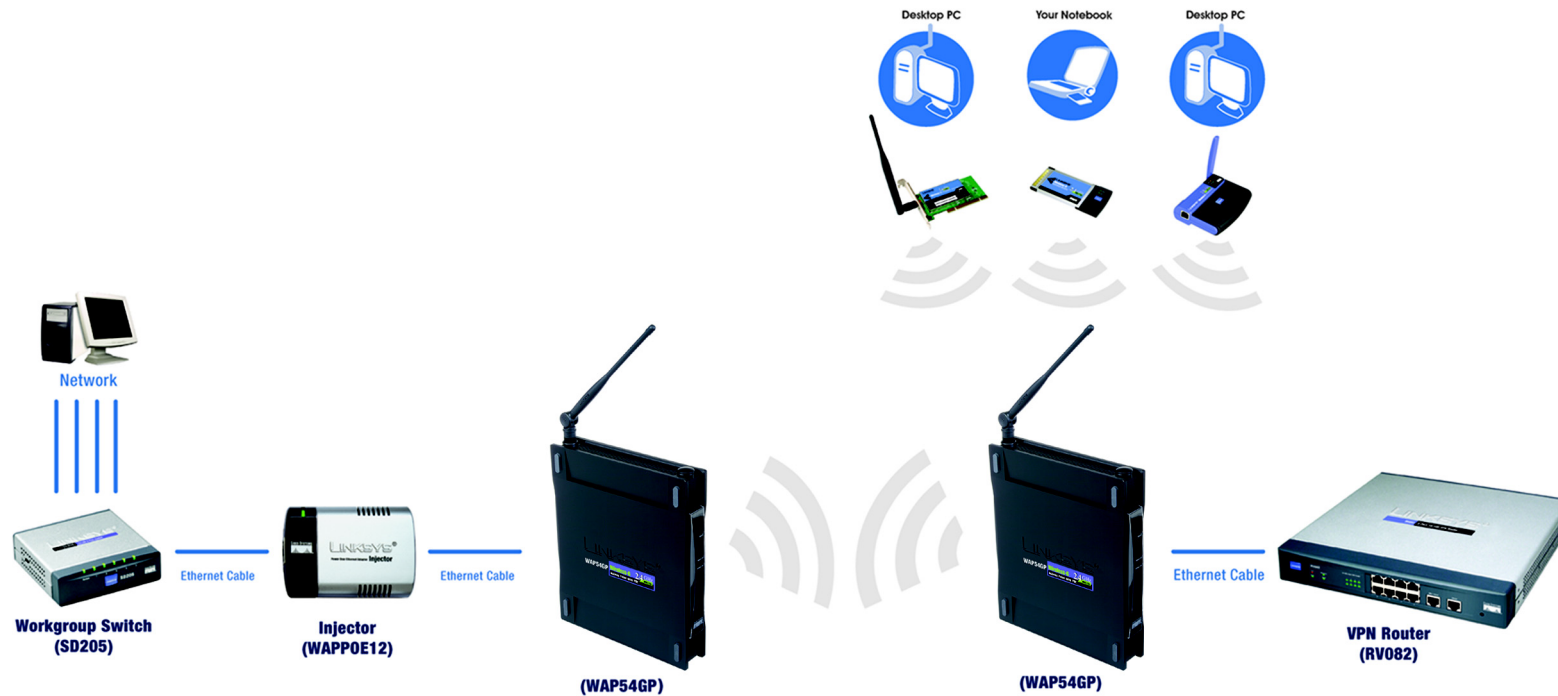
Figure 6-13: Wireless Repeater Diagram
