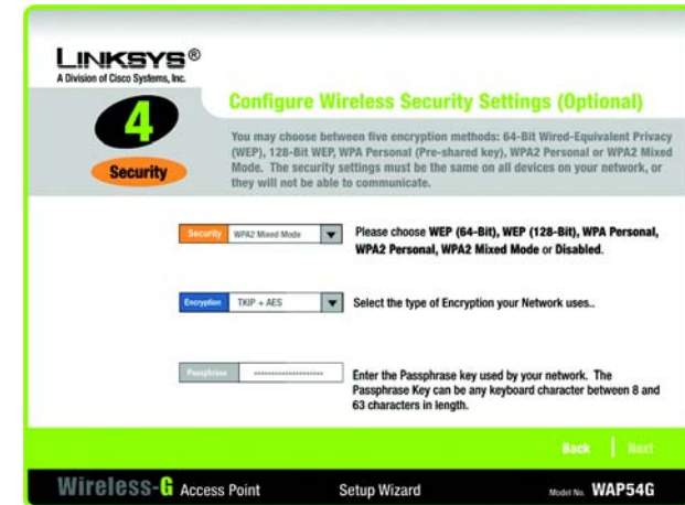
Figure 5-23: WPA2 Mixed Mode Settings Screen
