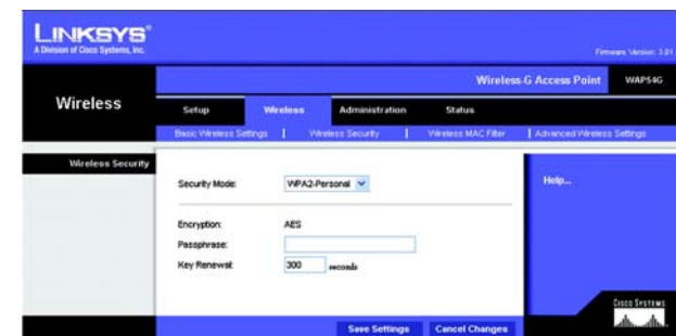
Figure 7-14: Wireless Security - WPA2-Personal Screen
