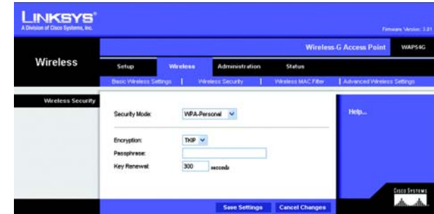
Figure 7-13: Wireless - Wireless Security (WPA-Personal) Screen
