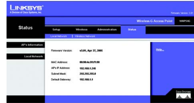
Figure 7-27: Status - Local Network Screen
