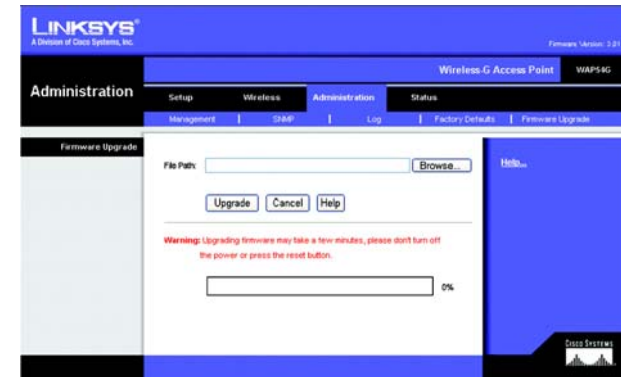
Figure 7-26: Administration - Firmware Upgrade Screen
