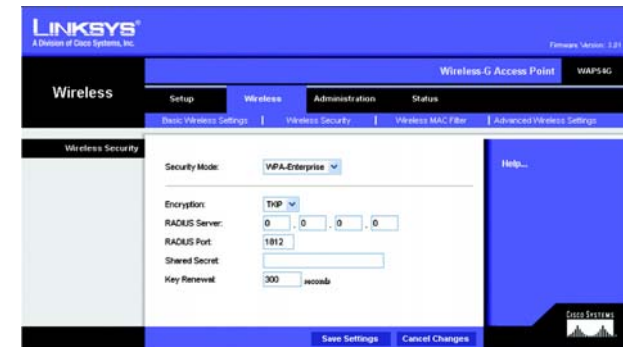
Figure 7-16: Wireless Security - WPA-Enterprise Screen
