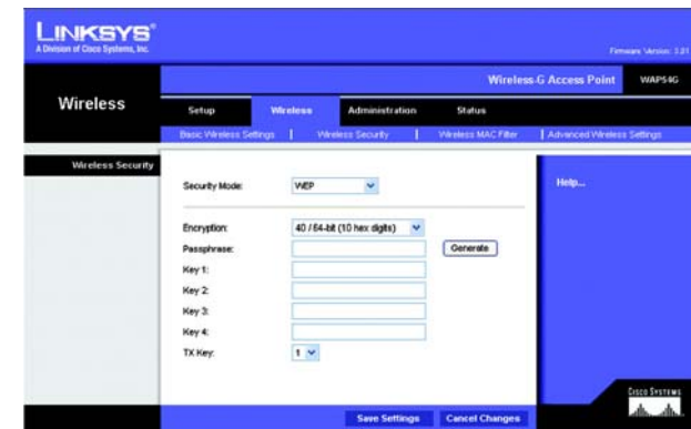
Figure 7-18: Wireless Security - WEP Screen
