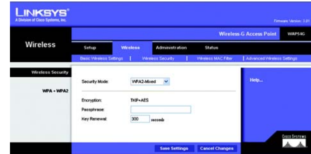
Figure 7-15: Wireless Security - WPA2-Mixed Screen
