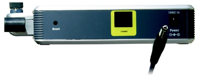
Figure 4-2: Connect the Power
