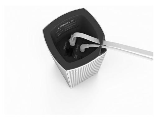
Internet port—Connect an Ethernet cable to one of the Gigabit (10/100/1000) ports, and to a broadband internet cable/DSL or fiber modem.
