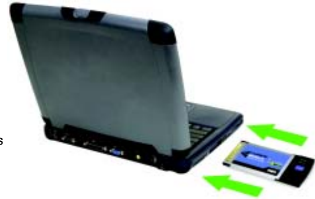
Figure 5-1: How the Adapter installs into your notebook
