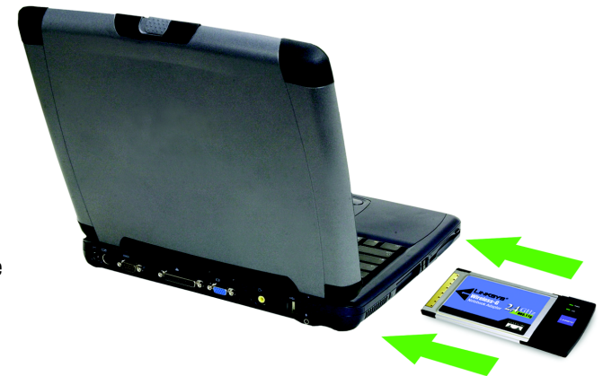
Figure 5-1: How the Adapter installs into your notebook
