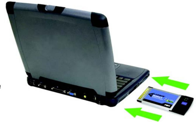
Figure 5-1: How the Adapter installs into your notebook
