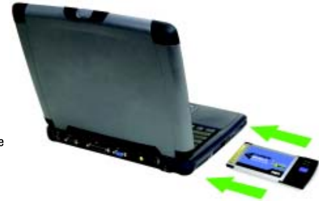
Figure 5-1: How the Adapter installs into your notebook
