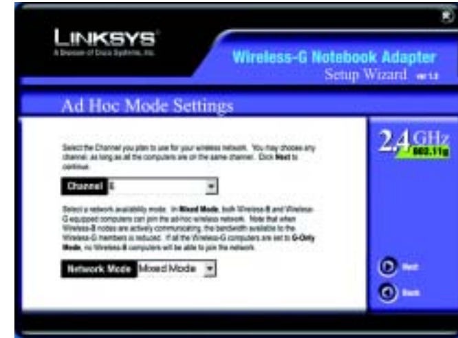
Figure 4-4: The Setup Wizard's Wireless Channels screen
