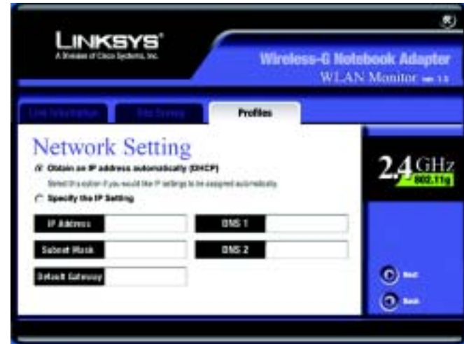
Figure 6-13: Network Setting for New Profile
