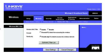
Figure 5-25: Wireless Tab - Wireless MAC Filter
