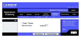
Figure 5-36: Applications and Gaming Tab - DMZ
