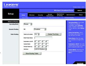
Figure 5-17: Setup Tab - Advanced Routing (Router)
