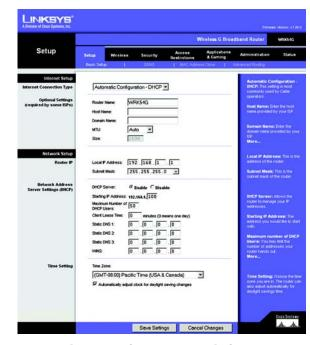
Figure 5-2: Setup Tab - Basic Setup
