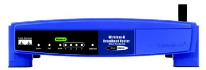
Green. The **Power** LED lights up and will stay on while the Router is powered on. When the
