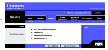
Figure 5-28: Security Tab - Firewall
