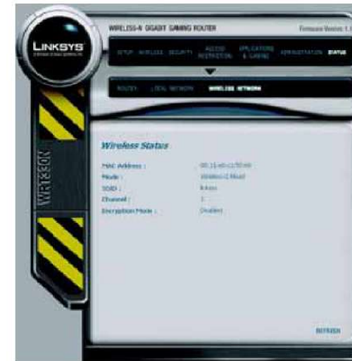
Figure 5-41: STATUS Tab - WIRELESS NETWORK
