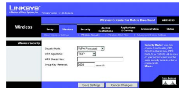
Figure 8-20: Wireless Tab - Wireless Security (WPA Personal - TKIP)
