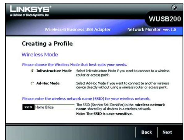
Figure 5-13: Creating a Profile - Manual Setup - Wireless Mode
