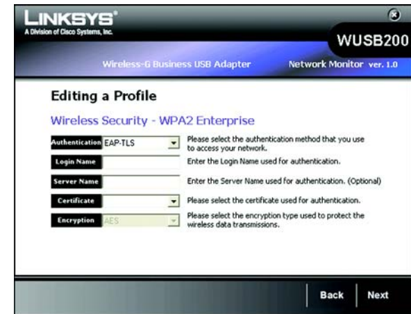
Figure 5-36: Editing a Profile - Wireless Security - WPA2 Enterprise - EAP-TLS
