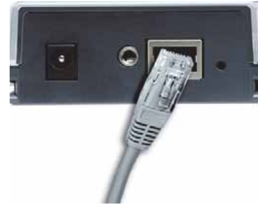
Figure 3-1: Connect the Ethernet Network Cable
