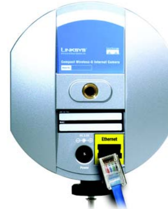
Figure 4-1: Connect the Ethernet Network Cable
