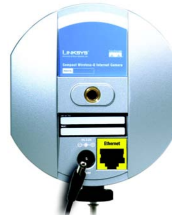
Figure 4-2: Connect the Power Adapter
