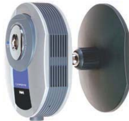
Camera in Wall-Mounting Position
