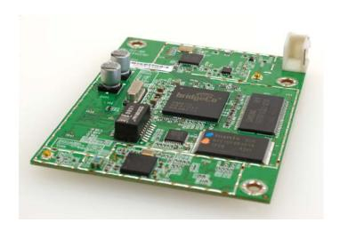
Complete audio networking system on a small module
