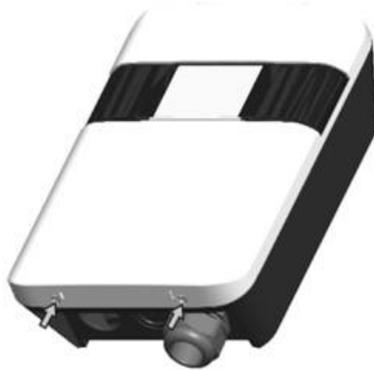
Figure 3-1 Loosen 2 Pcs M4 Screw
