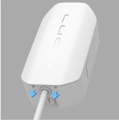
2. Slide logo cover up and remove by pulling from charging station housing.
