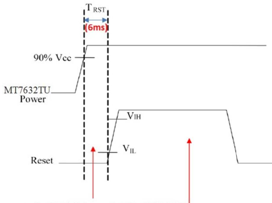
Keep Reset under  $V_{IL}$  (0.6V) over 6mS for MT7632TU
