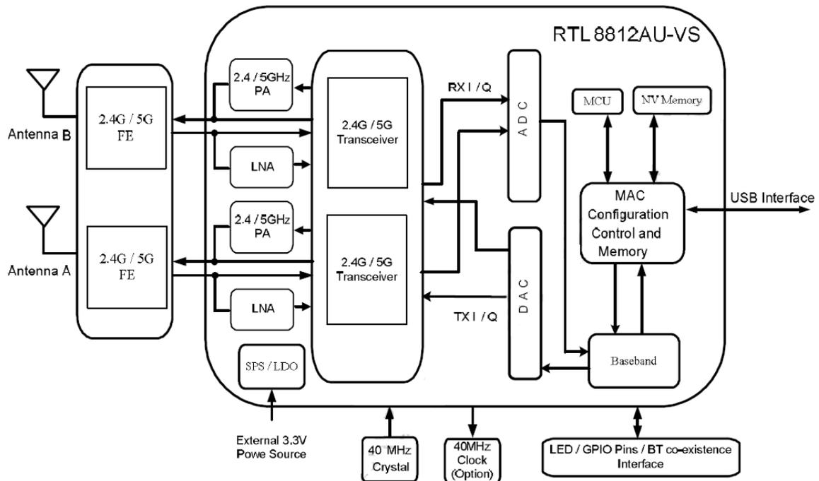
Figure 1. Dual-Band MIMO 2x2 Solution – RTL8812AU-VS (11ac 2x2 MAC/BB/RF + PA)
