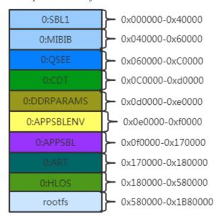
WiFi RF calibration data and MAC addresses are stored in "0:ART" partition, which is written during manufacturing process. Normally, we don't' need to modify the data in this partition.
