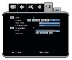
This is the general "SOURCE" layout which can be seen when selecting "SOURCE" in the on screen display (OSD).
