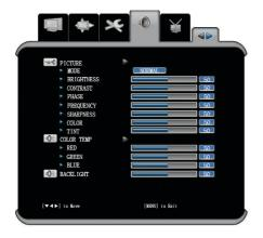
This is the general picture layout which can be seen when selecting "PICTURE" in the on screen display (OSD).
