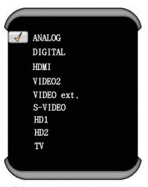
This screen is displayed when "SOURCE" button is pressed.
