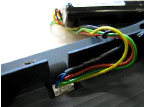
Figure 9.2 Disconnecting the battery wires from the minicare analyzer
