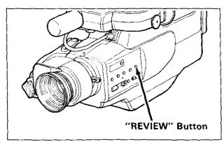
2. When the tape reaches the end of the scene you have just recorded, the Video Camera/Recorder returns to the record/pause (stand-by) mode. Recording starts again when the Record Start/Stop Button is pressed again.
