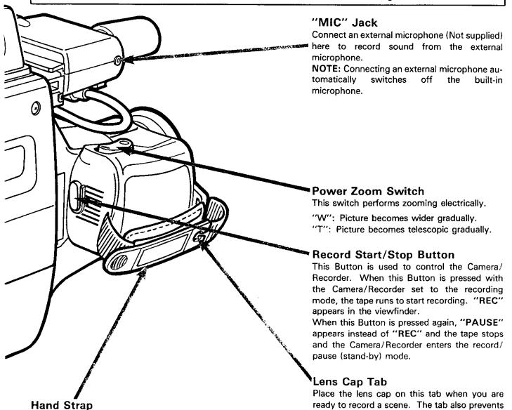
the lens cap from swinging around on its cord.
