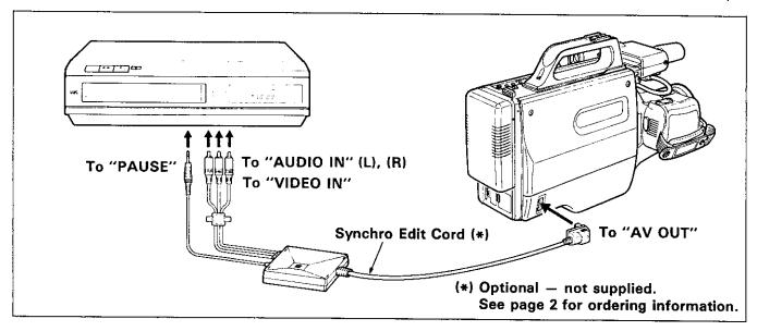
Connect your Camera/Recorder to a compatible VCR as shown above. An optional synchro edit cord is required.
