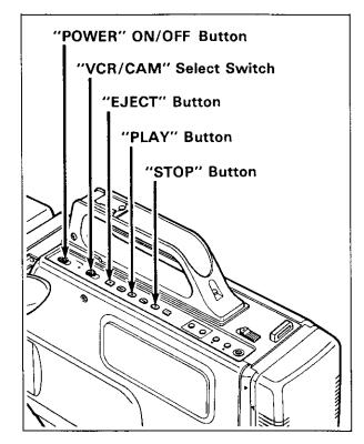
NOTE: If you want to watch a TV program with Video Camera/Recorder connected as illustrated, press "POWER" ON/OFF Button of the Video Camera/Recorder off, or disconnect the connector cable of RF Converter Unit from "AV OUT" jack on the Video Camera/Recorder.
