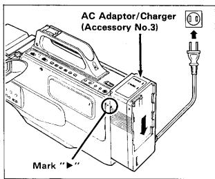
To remove slide the AC Adaptor/Charger upward while pushing the "BATTERY" Eject Lever in the direction of the arrow.
