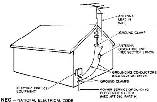
Power Lines—An outside antenna system should not be located in the vicinity of overhead power lines or other electric light or power circuits, or where it can fall into such power lines or circuits. When installing an outside antenna system, extreme care should be taken to keep from touching or approaching such power lines or circuits as contact with them might be fatal. Installing an outdoor antenna can be hazardous and should be left to a professional antenna installer.
