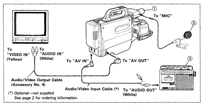
NOTES: • Sound from the built-in microphone, external microphone and the AV IN jack can be dubbed.
