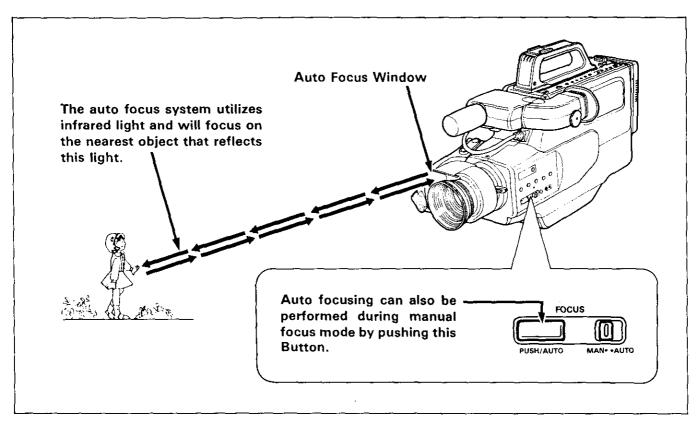
With the "FOCUS AUTO/MAN" Switch set to "AUTO" position, ordinary objects are automatically in optimum focus.
