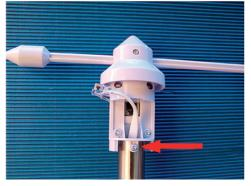
Insert the foot into the pipe and rotate it in such a way that it can be locked in the respective holes in the pipe using the two screws
