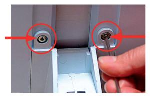
Screw the foot support on to the weather station using the enclosed Allen key and 2 Allen screws.
