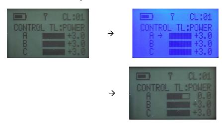
To select a zone, press the associated zone key, A/B/C. Pressing it once selects the zone and the arrow key will appear to the right of the selected zone (and power can be adjusted while the arrow key is present). To turn off a zone, press the associated A/B/C key twice.
